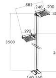
200 x 582 x H3500mm Palo/Pole Dimens. 80 x 40mm
