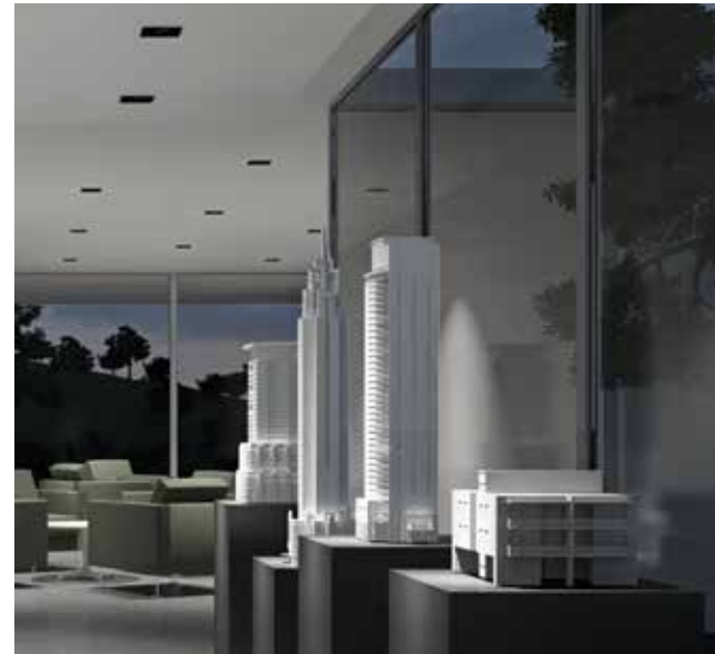
Accent Lighting 14^\circ < \alpha < 25^\circ Narrow beam to direct the attention to the object
